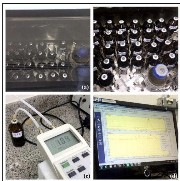
Figure 2.3 Methane production monitoring: (a) and (b) incubation; (c) pressure measure; and (d) area extraction for volume of methane estimation.
