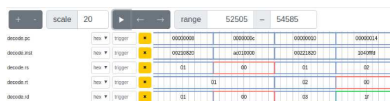
Figura 3.4: Monitoring five signals in the waveform window.
