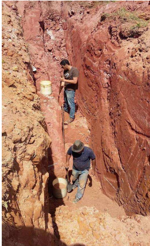
Figure 5.2: Collection of undisturbed samples at two depths and carried out inside a trench.
