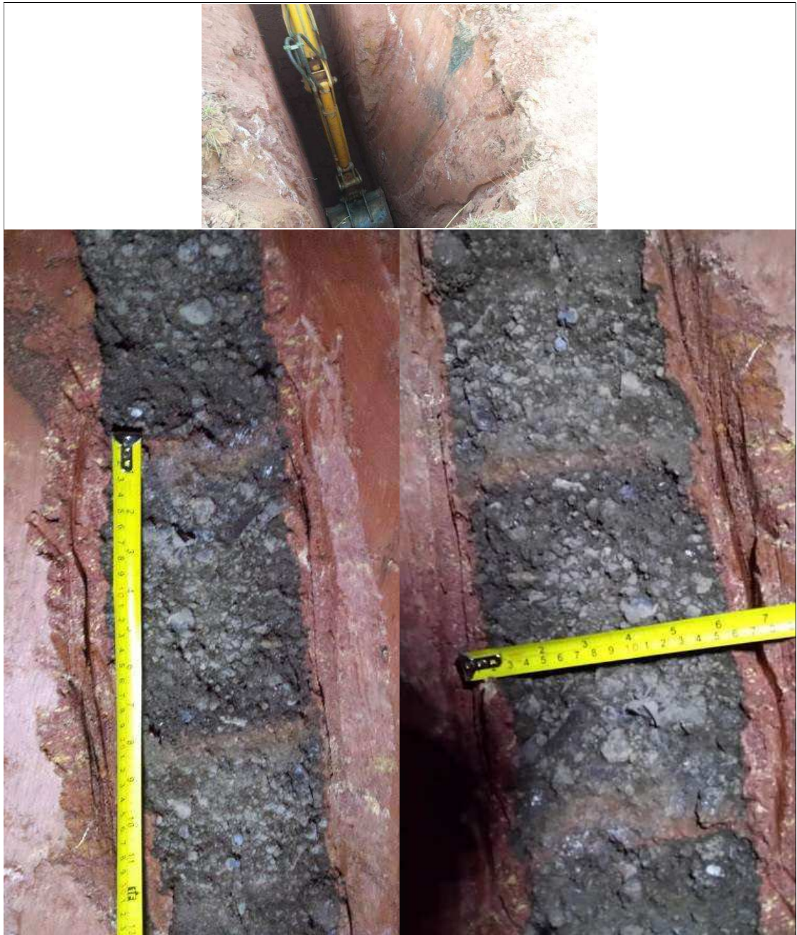
Figure 5.9: Results of the visual survey carried out on the Mini-RAP pile #4.
