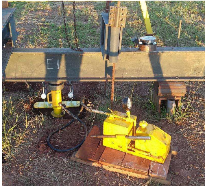
Figure 5.6: Load test performed using hydraulic jack, kneecap, measured with comparator watches and reacted with reusable anchor.
