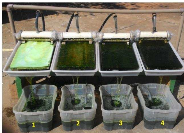
Fig. 1. System of reactors for the attached biomass growth in different support materials: (1) control reactor; (2) nylon; (3) polyester; (4) cotton.
