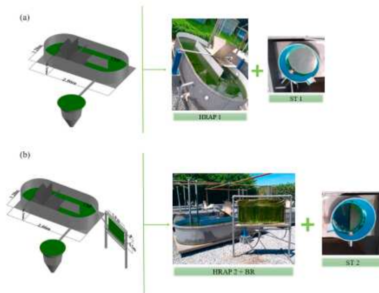
Fig. 1. Scheme of wastewater treatment and biomass production systems: (a) System 1, composed of HRAP and settling tank (ST1); (b) System 2, composed of HRAP, BR (in the photo BR with \alpha = 90^\circ ) and settling tank (ST2). The angle \alpha in the BR indicates the variation in panel inclination during the experiment.
