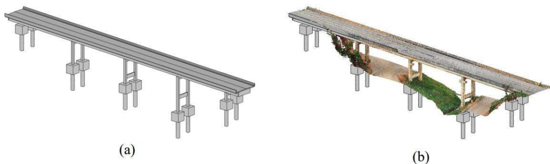
Figure 3. (a) proposed bridge model; (b) overlay of the model with the point cloud [31].
