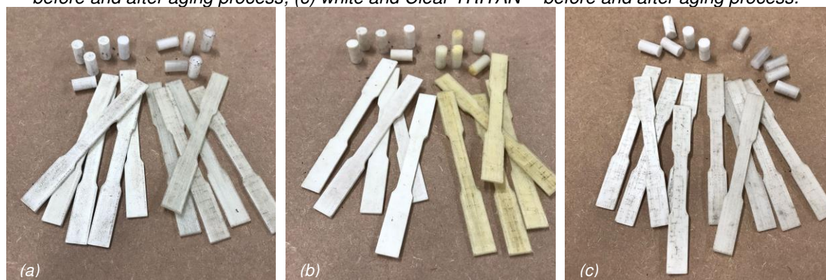
Figure 12: (a) White and Clear PETG before and after aging process; (b) white and Clear ASA before and after aging process; (c) white and Clear TRITAN™ before and after aging process.
