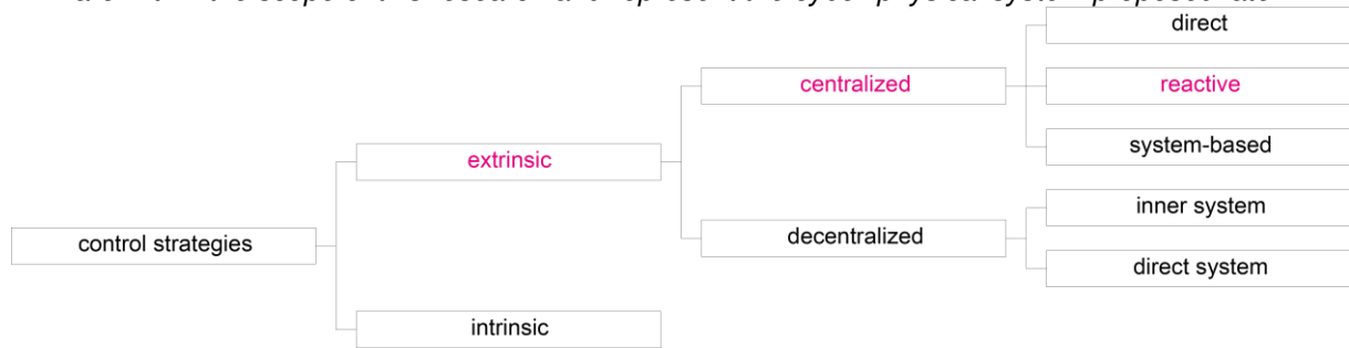
Figure 6: Controlling techniques: centralized and decentralized strategies. The solutions in magenta are within the scope of this research and represent the cyber-physical system proposed later.
