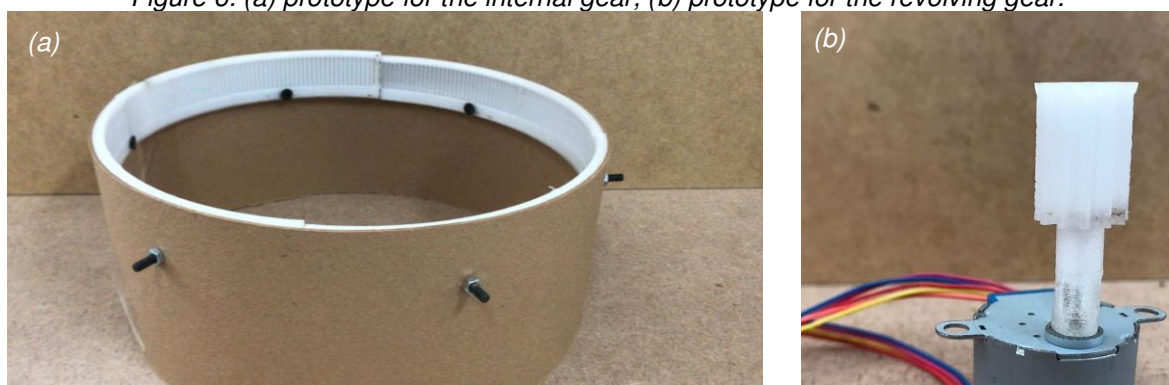
Figure 6: (a) prototype for the internal gear; (b) prototype for the revolving gear.
