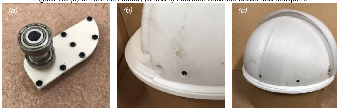
Figure 13: (a) tilt axis connector; (b and c) interface between shells and marquee.
