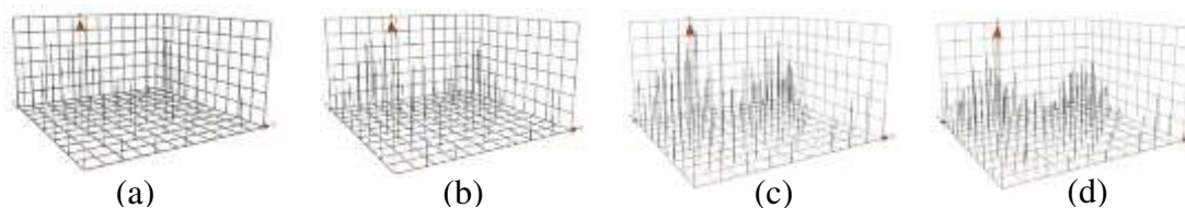
Figure 5 - Three-dimensional sampling figure of the quadratic regular grid of the altimetric survey in a section of “Zona da Mata” in the municipality of Viçosa, Minas Gerais State, Brazil. The grids displayed (a) 48 points, (b) 64 points, (c) 90 points, and (d) 110 points.
