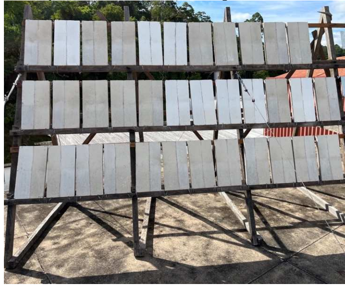
Figure 3.6- Paints exposed to the natural weathering resistance test for twelve months.
