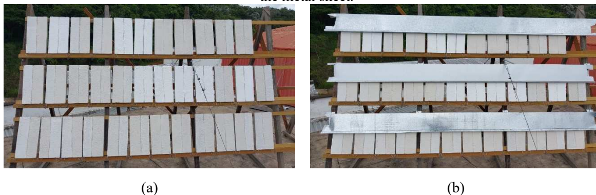
Figure 3.3- Weathering resistance test of paint samples: a) before fixing the metal sheet; b) after fixing the metal sheet.
