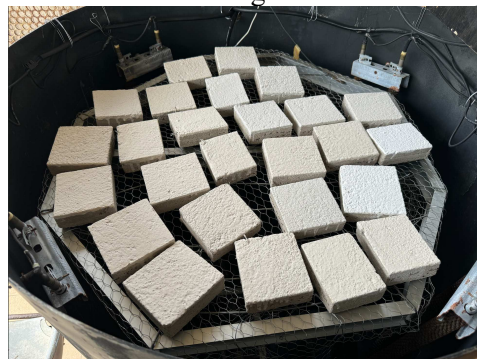
Figure 3.5- Accelerated weathering resistance test of paint samples.
