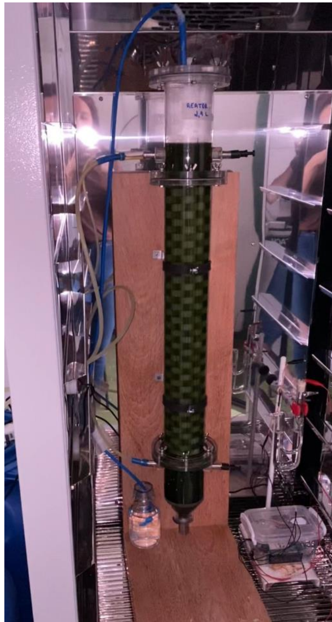
Figure 4.1 - Overview of the anaerobic structured-bed reactor (AnSTBR) used in the experiments
