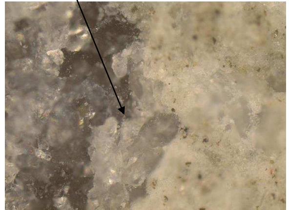
Figura 4.16 - Concreto com RMT – 200x (C5)
