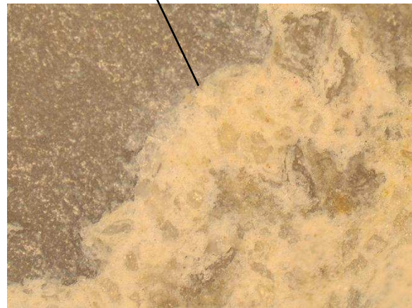
Figura 4.20 - Concreto com AMN e RCD – 100x
