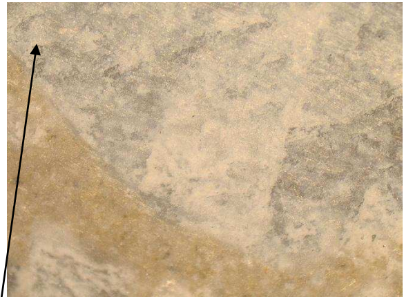
Figura 4.18 - Concreto com AMN e RCD – 100x
