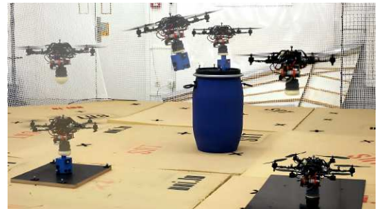
(b) The UAV resting on the gripper takes off and picks up the payload in blue presented in (KREMER et al., 2023).
