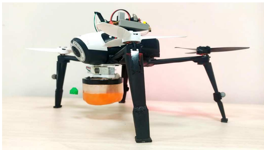
(b) Spraying system mounted on the UAV.
