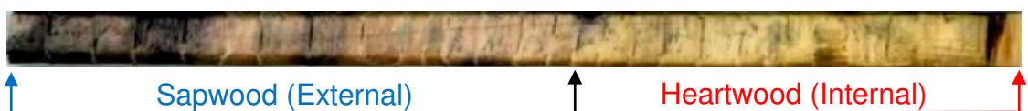
Figure 4.2. Photography of Avicennia wood sample with 9.2 cm length, 33 tree-rings/years old, and the accumulated tree-rings length
