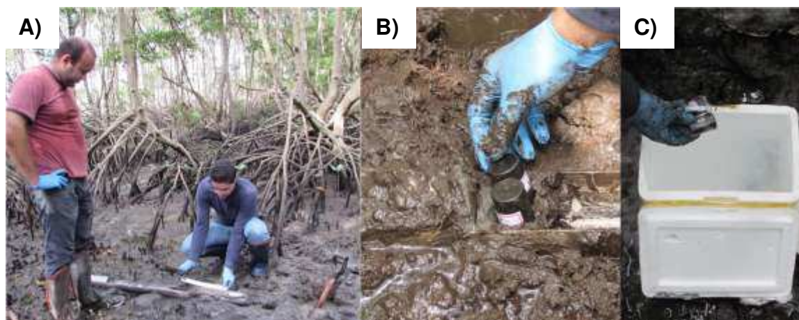
Figure 2.2. Soil sampling. A) Soil profile removed from the mangrove site and marked each 5 cm. B) Two plastic cups into the 5 cm wide soil layer to soil sampling. C) Closed and filled with soil samples plastic cups were placed in the box filled with liquid nitrogen immediately after collected.
