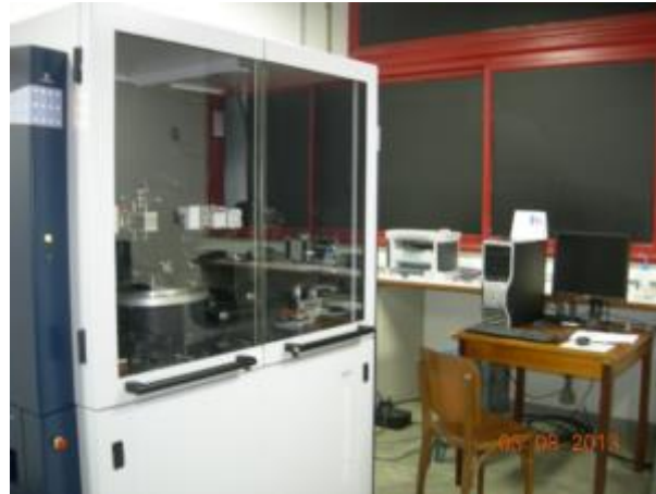
Figure 3-17. D8 Discover, available in the Laboratório de Difração e Espalhamento de Raios-X at the Department of Physics in UFV. Adapted from the Website from Physics Department at UFV access by the link http://www.posfisica.ufv.br/?page_id=81#ER .
