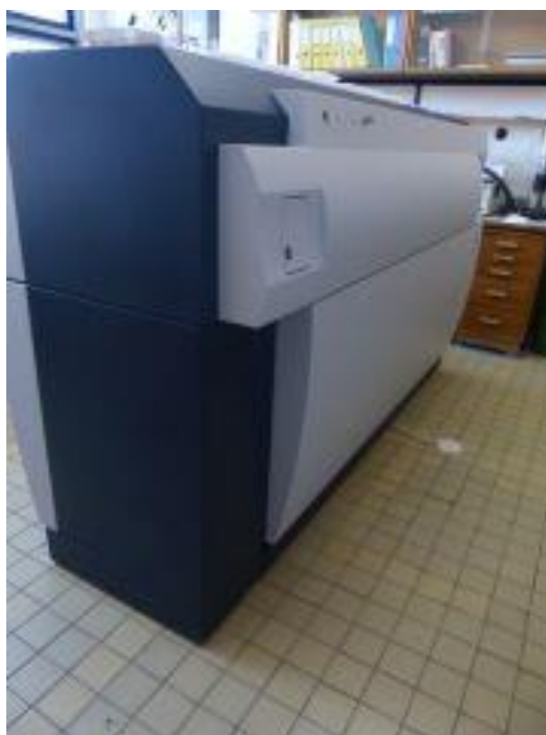
Figure 3-20. MALDI-TOF/TOF mass spectrometer UltrafleXtreme, manufactured by Bruker Daltonik and available at the Institute of Macromolecular Chemistry (Czech Academic of Science). Adapted from the Website from Institute of Macromolecular Chemistry access by the link https://www.imc.cas.cz/en/research/research-departments/ .
