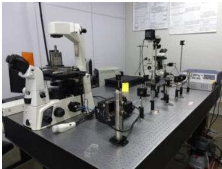
Figure 3-12. Optical Tweezers available in the Laboratório de Física Biológica on the physics department in the UFV. Adapted from the Website from Physics Department at UFV access by the link http://www.posfisica.ufv.br/?page_id=81#ER .
