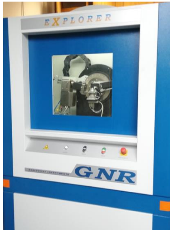
Figure 3-18. High-resolution diffractometer GNR Explorer (Italy) with a Mythen 1K strip detector available in the Institute of Macromolecular Chemistry (Czech Academic of Science). Adapted from the Website from Institute of Macromolecular Chemistry access by the link https://www.imc.cas.cz/en/research/research-departments/ .
