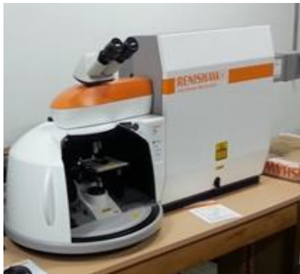
Figure 3-10. Equipment MicroRaman - Renishaw Invia is available at Laboratorio de Espectroscopia Raman in the Physics Department (UFV). Adapted from the Website from Physics Department at UFV access by the link http://www.posfisica.ufv.br/?page_id=81#ER .
