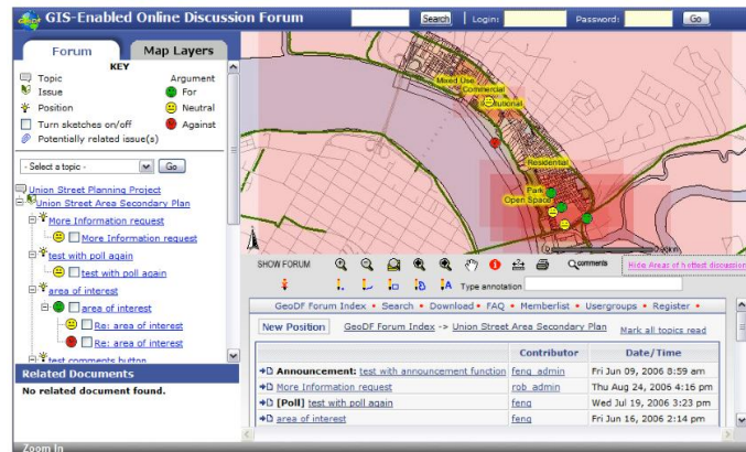
Figure 5 User Interface of spatial search for arguments (location of discussion contributions) and show hottest area of discussion
