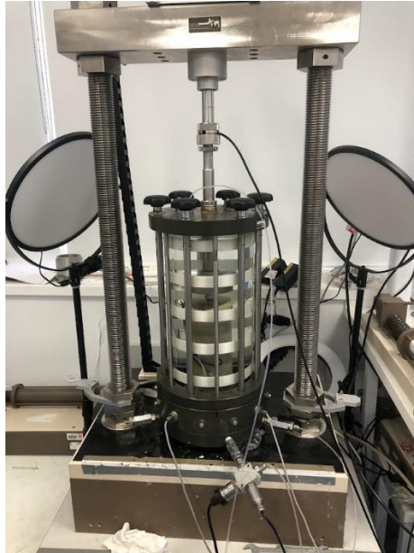
Figure 3.13. CSD test with shear wave velocity measurements.
