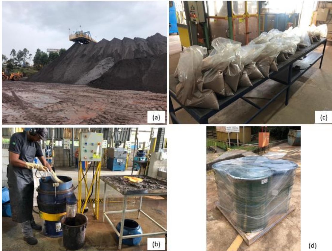
Figure 3.2. Sample preparation: (a) Collection at the processing plant; (b) Washing to separate fines; (c) Drying and storage in plastic bags; (d) Storage in metal drums for later transportation.
