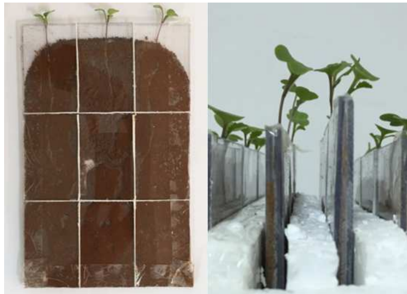
Figure 1. Transparent acrylic plates designed to create a system for visualizing root growth.
