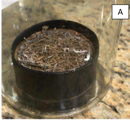
Figure B2 — Soil cylinder inside the glass jar during the incubation (A); Remaining root litter at the end of incubation (B); Detail of the cylinder slicing device and the measurement of the layer with a pachymeter (C); Slicing of the soil cylinder with a razor (D).
