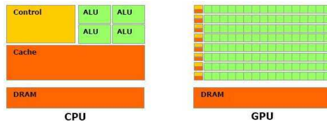
Figure 3.2: Comparison between GPUs and CPUs structures. Source: [NVIDIA, 2014]
