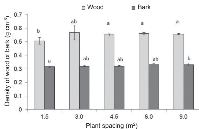
Figure 1 Mean basic densities of wood and bark in Eucalyptus trees planted at different spacings; means with the same letter are not significantly different (Tukey test, p > 0.05 )
