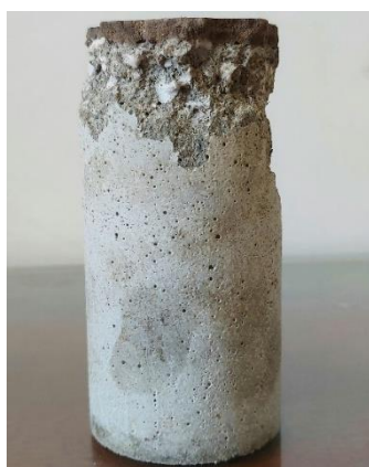
Figure 4.7 – specimen ruptured in the compressive strength test.
