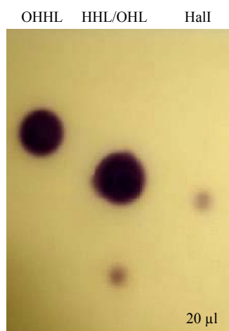
Figure 29 - A representative thin-layer chromatogram of Hall expression in E. coli XL1-Blue cultured in ABG minimal medium. Spots were detected with C. violaceum CV026 reporter strain. Standards: N-(3-oxohexanoyl)-L-homoserine lactone (OHHL); N-(hexanoyl)-L-homoserine lactone (HHL); N-(octanoyl)-L-homoserine lactone (OHL); (Hall) E. coli XL1-Blue harbouring pQE-30Xa-hall.
