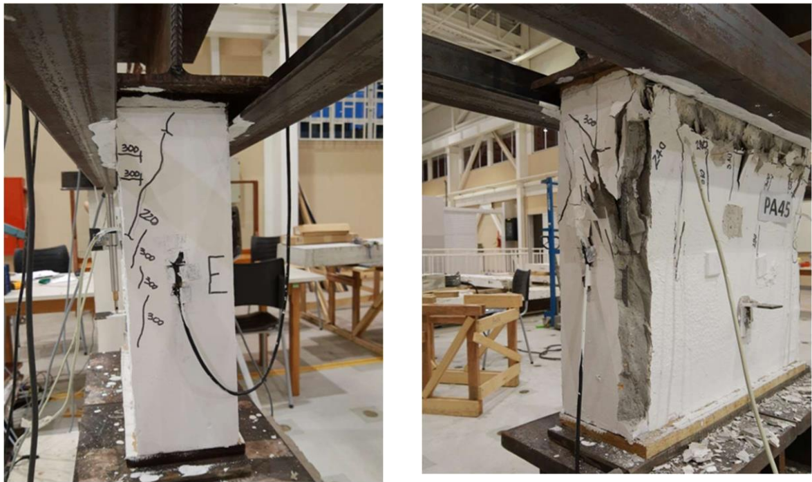
Figure 3.11 - PA4 sandwich panel failure.
