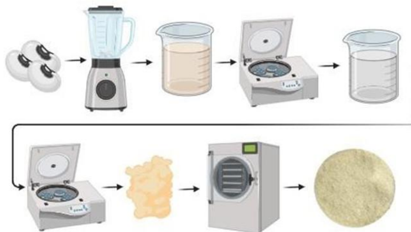
Figure 1. Flowchart of the white bean protein concentrate extraction process. The steps include grinding the beans in a blender (initially on the left), adjusting the pH to 10, centrifugation for fraction separation, subsequent pH adjustment (to 3), a second centrifugation to obtain the precipitated protein, and finally drying the protein concentrate, resulting in a powder.
