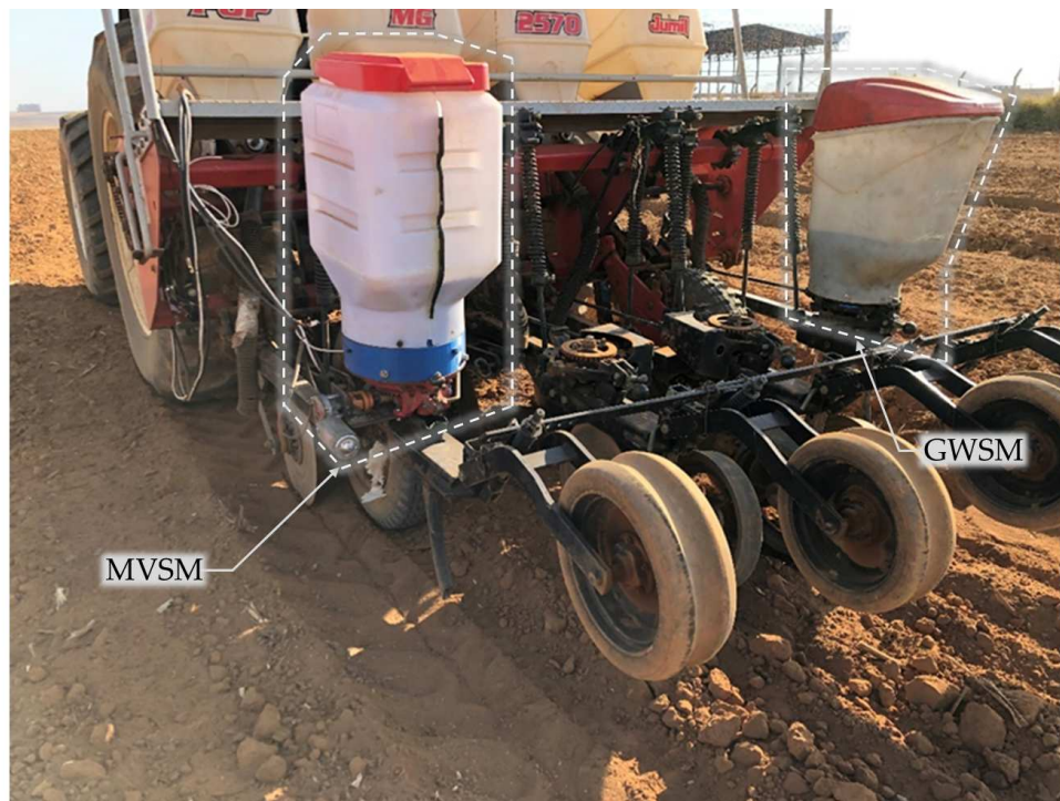
Figure 13 – MVSM and GWSM installed on the planter's outer rows
