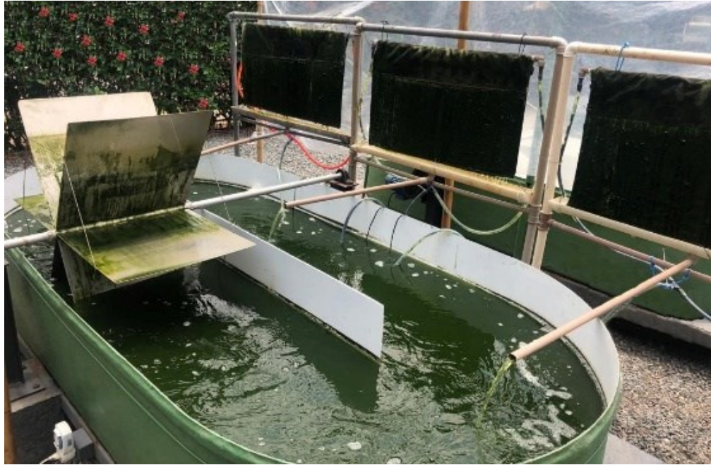
Figure S5.1. BRs integrated into a HRAP, composing the hybrid system.
