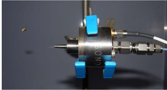
Figure 2: The ultrasonic nozzle system used in the wind tunnel and the flying response of a male Sitotroga cerealella .
