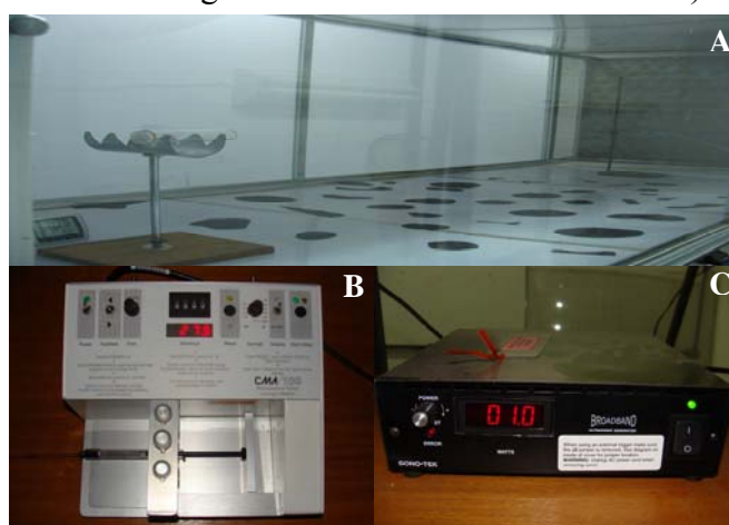
Figure 1: A wind tunnel with piezoelectric sprayer was used in this experiment; A. wind tunnel, B. microinjection pump (CMA/100) and C. ultrasonic generator.
