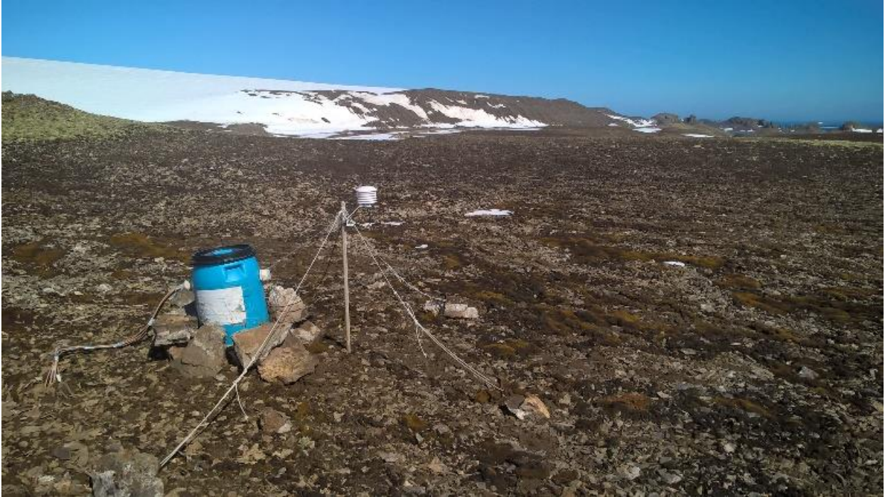
Figure 4 – Photography of the soil temperature and moisture CALM Sensor location of the monitoring site of the Terrantar / UFV / INCT project, in Stansbury peninsula, Nelson Island, maritime Antarctic.
