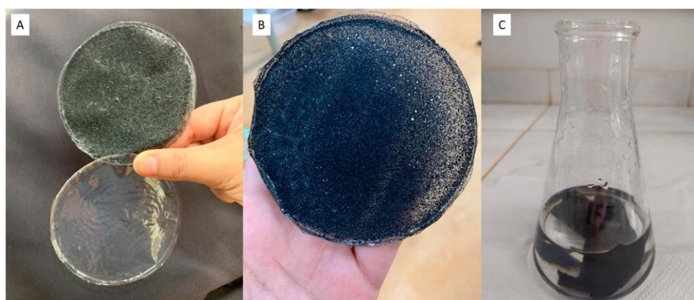
Figure 2. (A) Cellulose acetate film without (pure) and with bonechar; (B) cellulose acetate film with bonechar; (C) visualization of the attachment of the material to the film (translucent water after 24 h of agitation).
