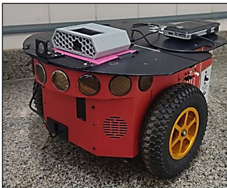
Figure 26 – Robotic system used: Pioneer 3-DX robot and Jetson Nano single-board computer.
