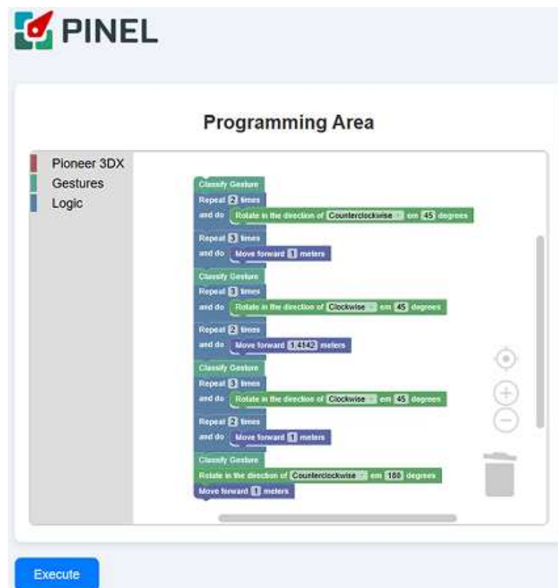
Figure 17 – Block program combining repetition loops with rotation and linear displacement commands.
