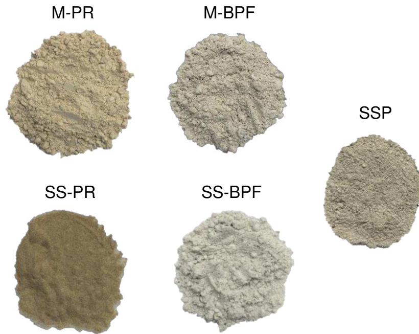
Fig. A2. Macroscopic appearance of Morocco (M) and Serra Salitre (SS) phosphate rocks before (PR) and after acidulation (BPF) with biogenic acid, and single superphosphate (SSP). BPF = biogenic P-fertilizer.
