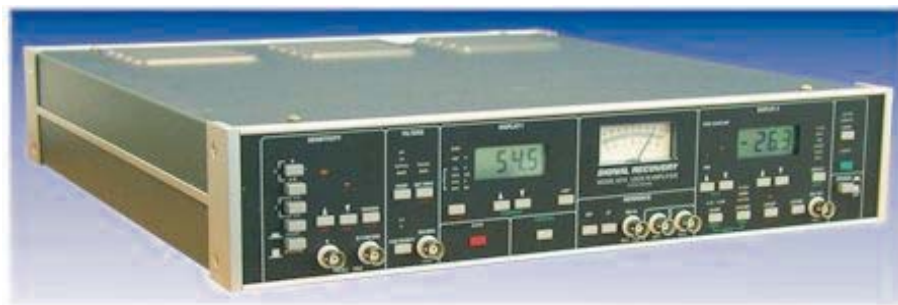
Figura 1.29: Amplificador lock-in: “Signal Recovery model 5210 lock-in Amplifier”.
