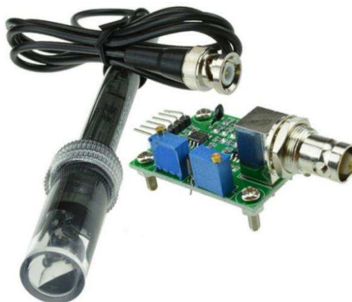
Figura 49. Módulo DIY MORE PH-4502C e sensor de pH E-201C
