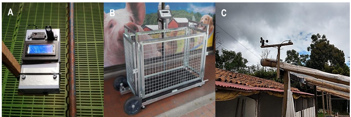
Figure 7. Equipment and data collection modules. (A) Internal module. (B) Weighing scale. (C) Outside module. Each internal module contained a camera that monitored males and females separately.
