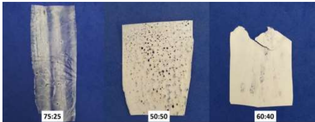
Figure S1. Cellulose acetate and zein blends prepared with different polymer ratios (wt/wt).
