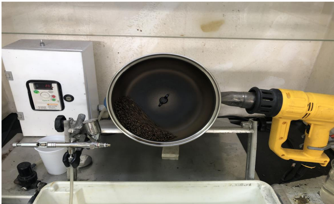
Figure 2: Granulator dish accompanied by heating gun and micro spray for fertilizer coating.
