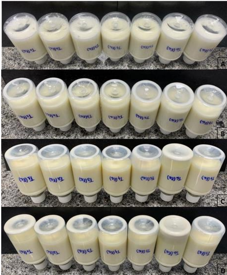
Figure 4. Gelation process of UHT milk samples throughout the shelf life. A: t = 0 h; B: t = 7 days; C: t = 15 days and D: t = 30 days. The process was similar in the three repetitions.
