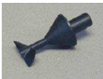
Figura 4. Sensor da Starch Pasting Cell
