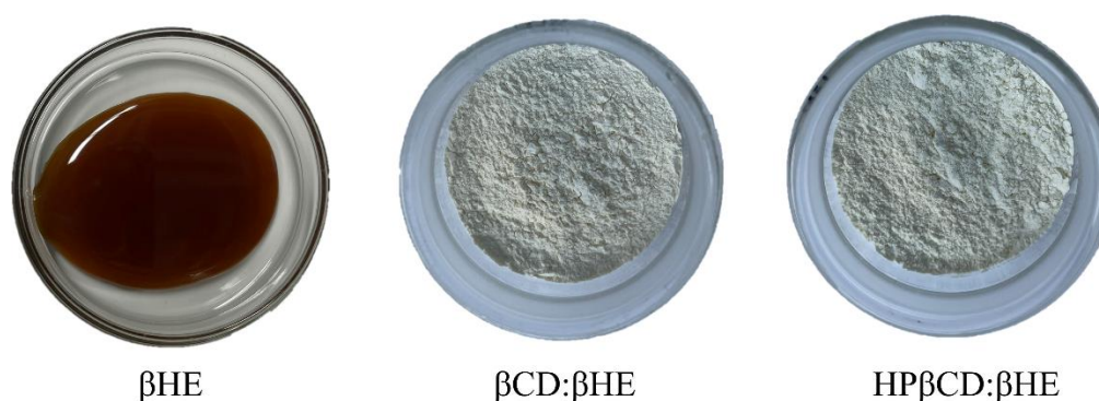
Figure 1. Physical appearance of the pure \beta HE and the obtained inclusion complexes \beta CD: \beta HE and HP \beta CD: \beta HE.
