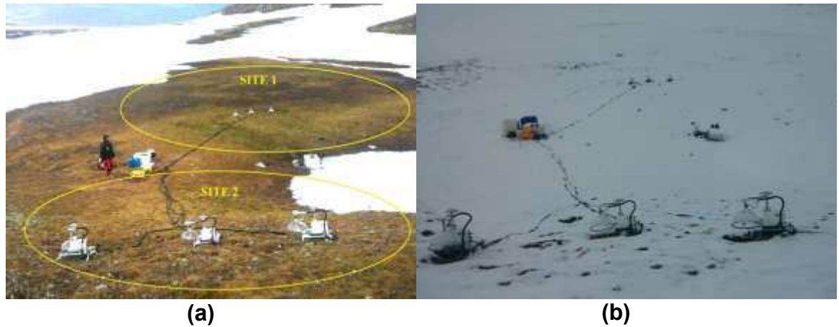
Fig 2. Illustrative images showing the system used to collect data of NEE and soil temperature in the studied sites in Coppermine Peninsula without (a), and with snow (b) covering the surface.
