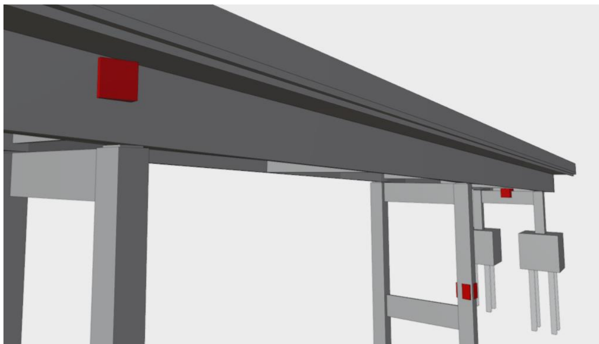
Figure 16. Generic damage geometrical representation identified by red cubes located in the damaged element's centroid.
