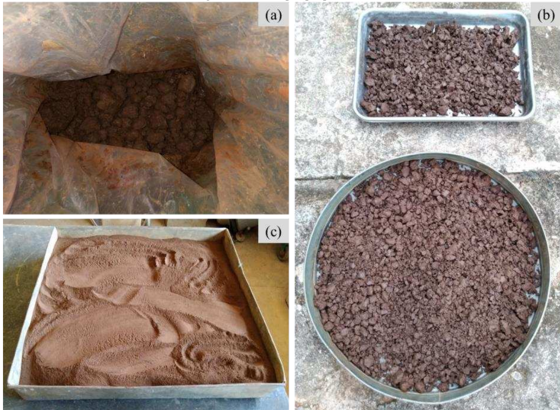
(a) Collected sample in a plastic bag; (b) Sample dried at room temperature; (c) Sample after loosening, sieving, and homogenizing. Source: elaborated by the author.
