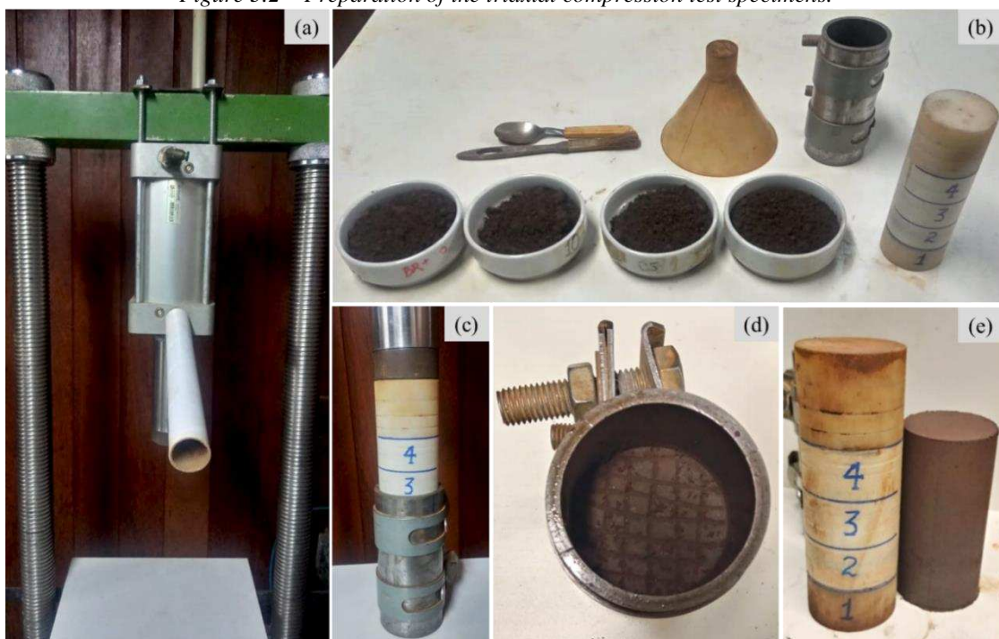
(a) Press used to compact the samples; (b) Equipment used and portions of material separated for each layer; (c) Specimen being compacted; (d) Scarified layer after its compaction; (e) Prepared specimen beside the cylindrical ruler. Source: elaborated by the author.
