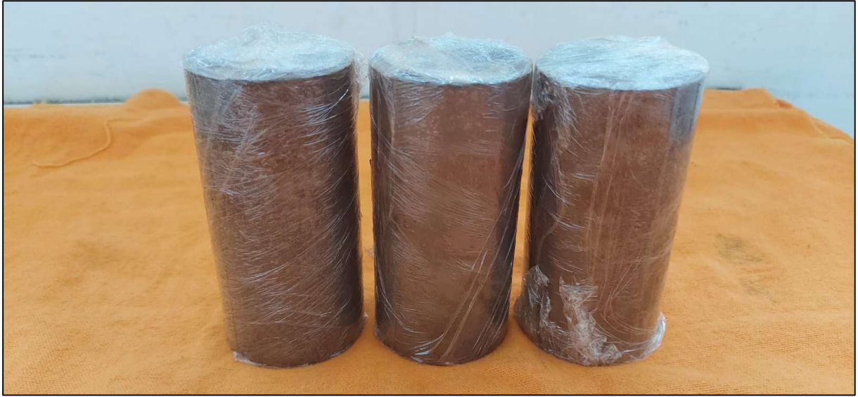
Fig. 3 Specimens molded for hydraulic conductivity tests ( \varnothing 50 mm \times 100 mm)
