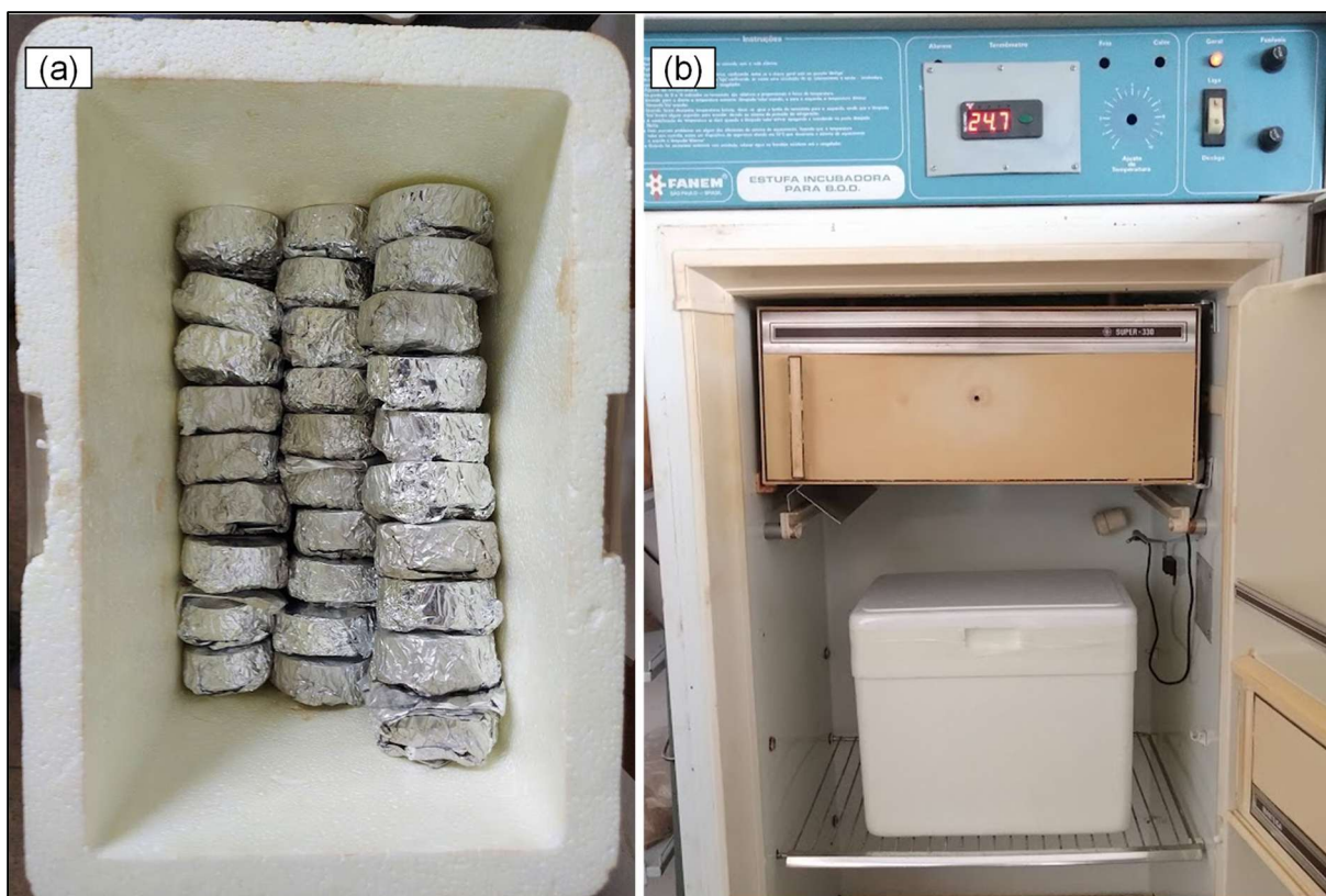
Fig. 6 Equilibration stage for the filter paper test. a specimen in sealed Styrofoam box; b temperature-controlled incubator set to 25 \pm 0.5 °C
