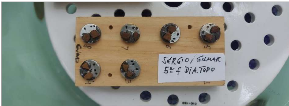
Fig. 4 Mounted specimens of IOT tailings fixed on 1 cm stubs with graphite-based adhesive for SEM/EDS analysis
