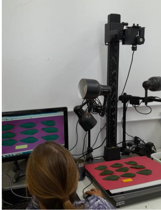
Figure 2. Setup assembled for capturing images of soybean ( Glycine max (L.) Merr.) leaflets at R5 stage.
