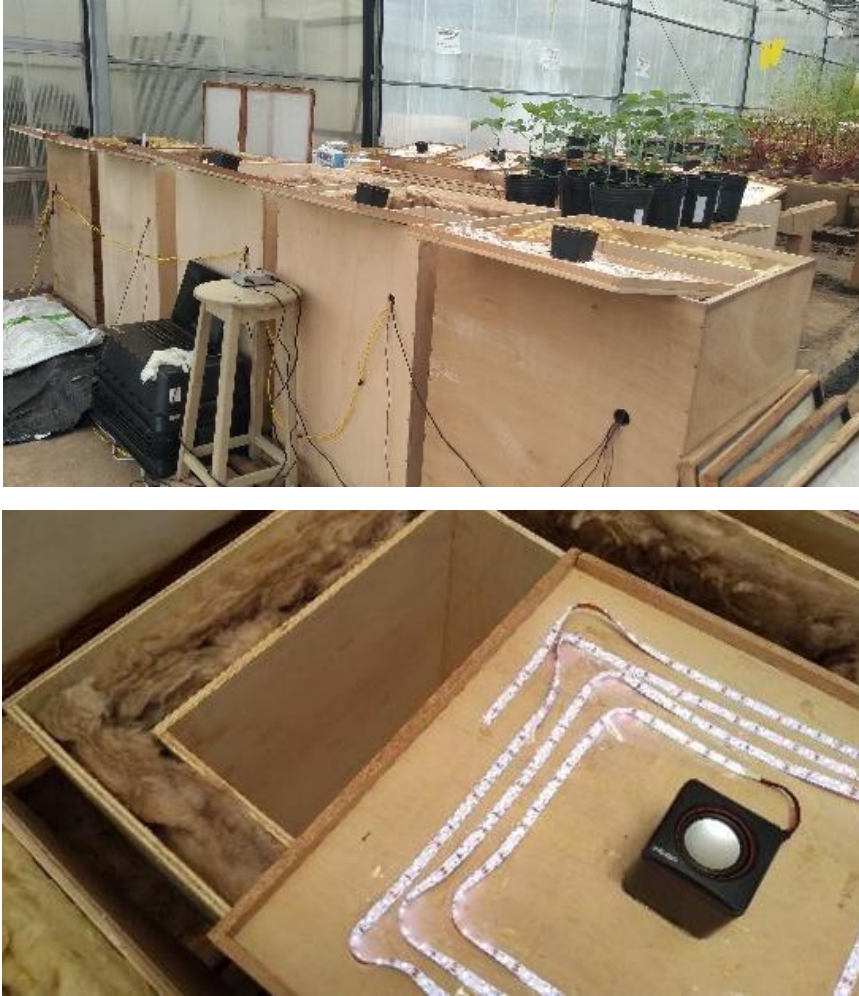
Figure S1. Acoustic treatment boxes equipped with a lighting and audio reproduction system.
