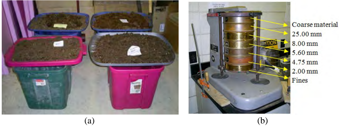
Figure 3.11 - As-received compost drying (a) and (b) shaker and sieves used to characterize particle size ranges.
