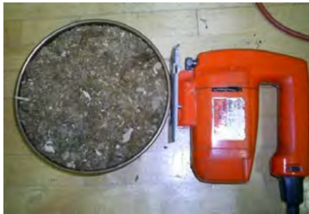
Figure 3.12 - Cylinder with compost bulking material vibrating.
