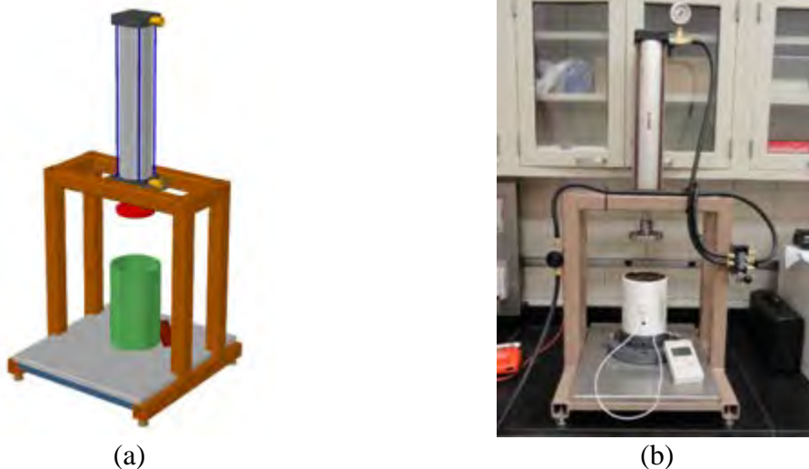
Figure 3.17 - Mechanical pressing device designed (a) and (b) constructed to provide different degrees of static and dynamic compaction.
