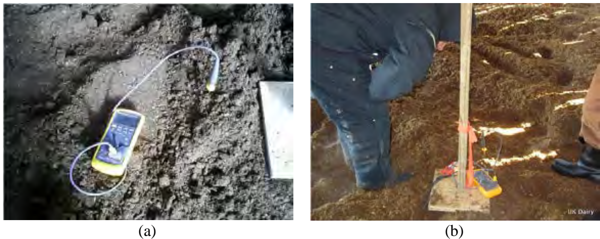
Figure 3.7 - Thermocouple-based thermometer used to measure bedding temperature.
