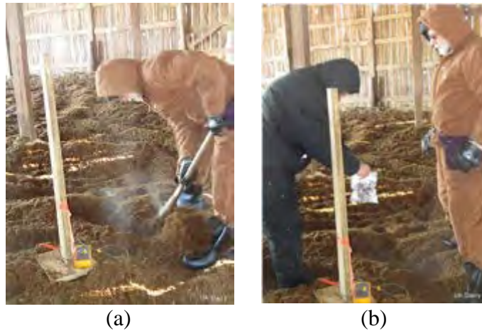
Figure 3.8 - Equipments used to collect the bedding sample: iron hoe (a) and (b) storage in plastic bags.
