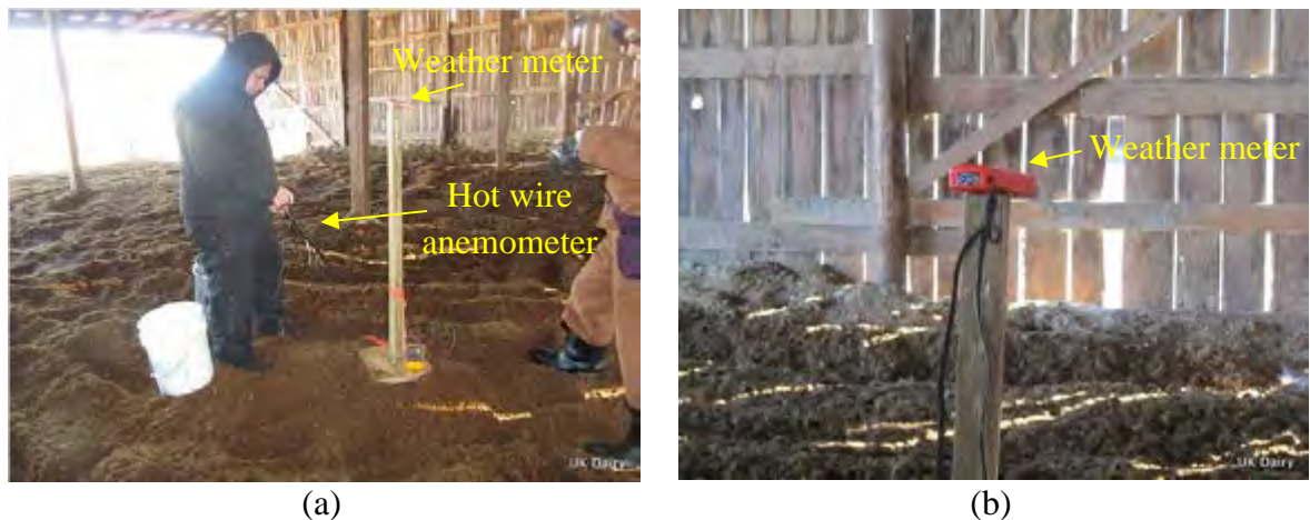
Figure 3.4 - Equipments used to measured environment: (a) hot wire anemometer and (b) weather meter.
