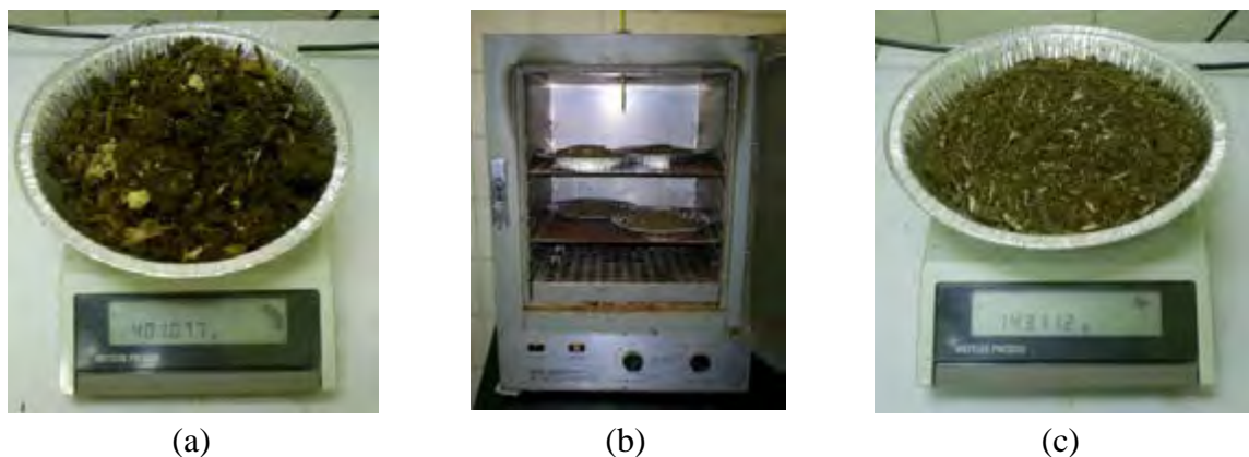
Figure 3.9 - Determination of moisture content in compost material: (a) wet weight of sample, (b) samples inside the oven, and (c) dry weight of sample.
