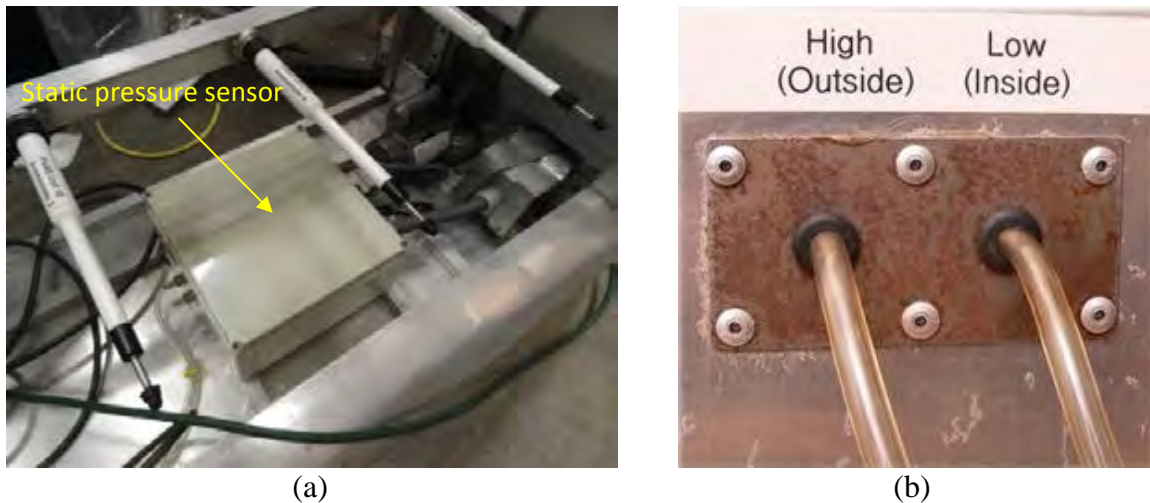
Figure 3.24 - Static pressure sensor (a) and (b) hoses on the sensor for static pressure measurement.
