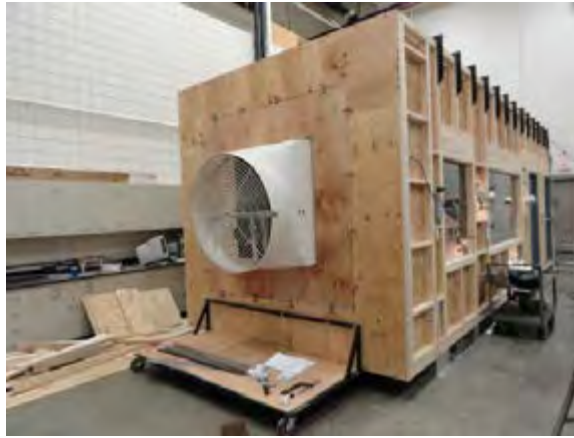
Figure 3.20 - View of the fan mounted on the wind tunnel.
