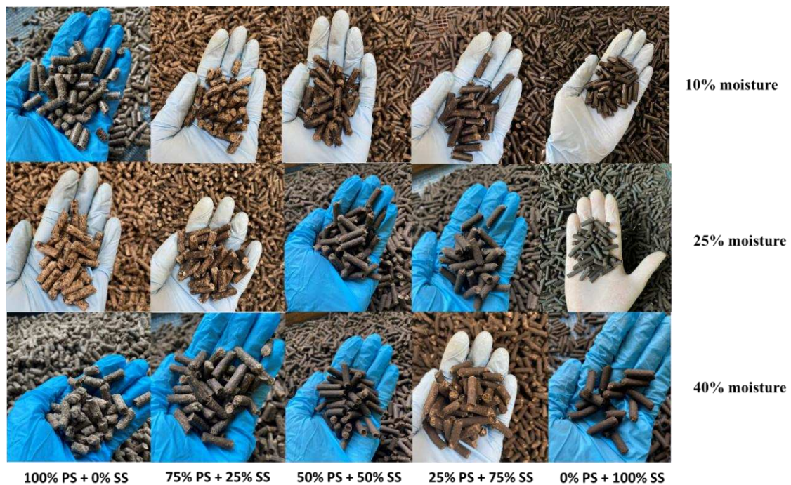
Figure 3.4. Pellets produced with different blends of primary (PS) and secondary sludge (SS) at 10%, 25% and 40% moisture content
