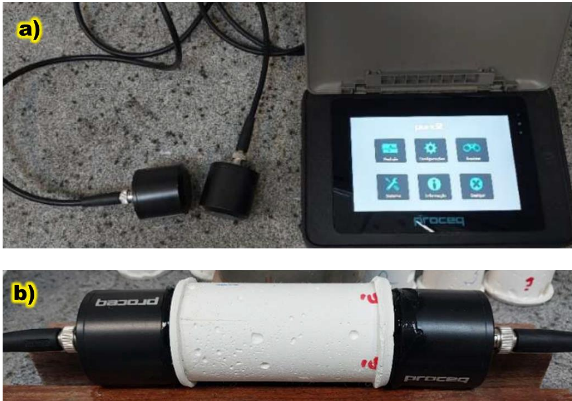
Figure 4-2 – Ultrasonic Pulse Velocity (UPV) setup: (a) Proceq Pundit Lab equipment; (b) UPV test being performed on a cylindrical gypsum-rubber specimen
