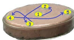
Fig. 3 Selected locations on the ground meat sample placed in a Petri dish for spectra acquisition. Center (1), top corner (2), bottom corner (3), left corner (4), and right corner (5)
