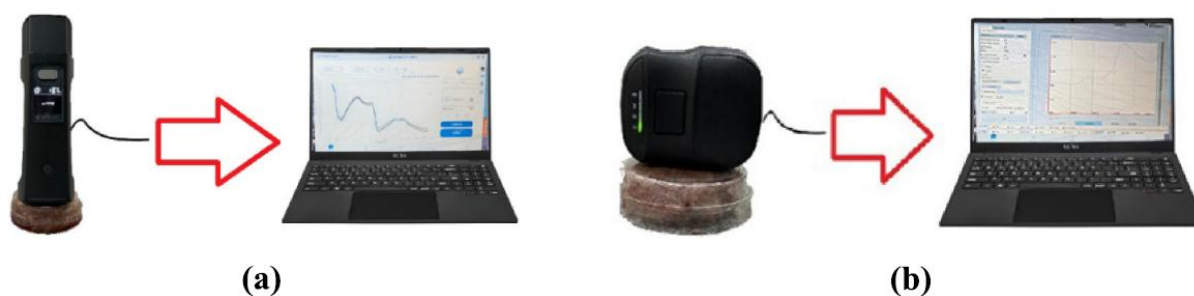
Fig. 2 Instruments set-up used to obtain the spectra of sous vide samples: a) NeoSpectra; b) InnoSpectra
