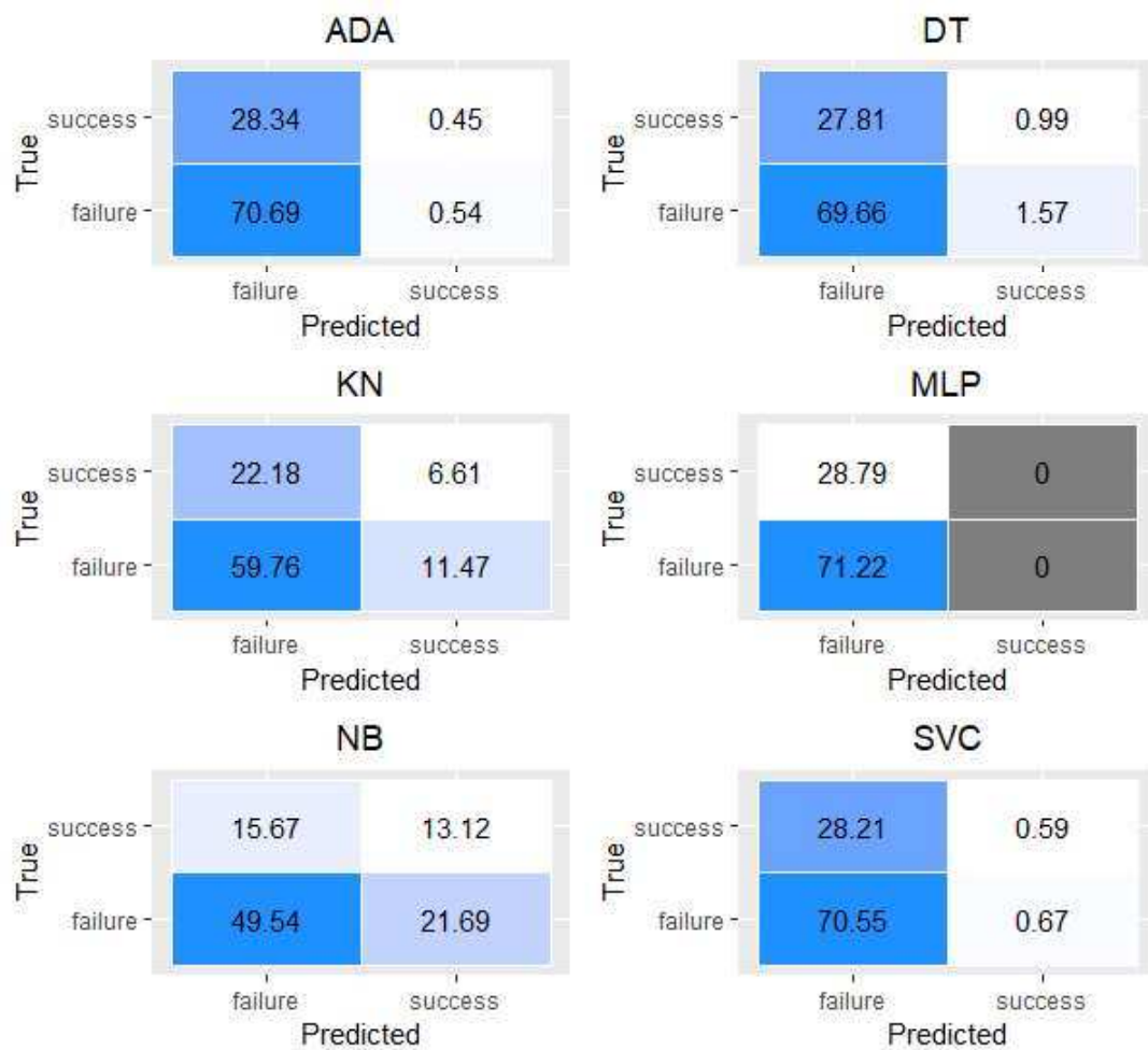
Figure 6. Confusion matrix in percentage for the failure and success classes predicted by machine learning classifiers (AdaBoost - ADA, Bernoulli Naïve Bayes - NB, Decision Tree - DT, Nearest Neighbors - KN, Multilayer Perceptron with one layer, one neuron and identity activation function - MLP and Support Vector Machine for Classification - SVC) from test sets with thousand markers.
