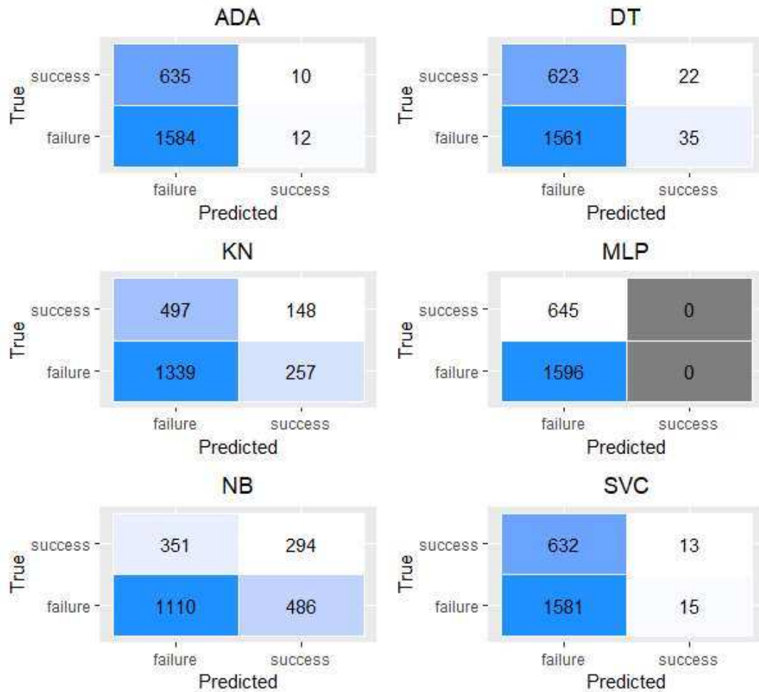
Figure 4. Average confusion matrix for the failure and success classes predicted by machine learning classifiers (AdaBoost - ADA, Bernoulli Naïve Bayes - NB, Decision Tree - DT, Nearest Neighbors - KN, Multilayer Perceptron with one layer, one neuron and identity activation function - MLP and Support Vector Machine for Classification - SVC) from test sets with thousand markers.
