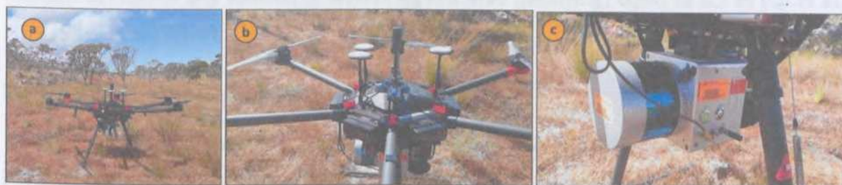
Fig. 3. GatorEye UAV-lidar (Gen 1) system. a) DJI M600 Pro hexacopter, with Phoenix Scout Ultra, hyperspectral, and visual sensors; b) three GNSS antennas for navigation, and one for sensor trajectory (positioned in the middle); c) Velodyne Ultra Puck lidar system.
